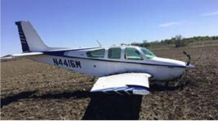
As many of you know, I made a forced, off-field landing last month in N4416W when the engine suddenly lost power in cruise flight. Upon landing in a plowed field, the nose gear collapsed, causing damage to the prop and engine cowling. While there are many lessons to be drawn from this experience, which is a longer conversation, the question I have been asked most often is: How do the NTSB 830 incident/accident reporting requirements work in practice?
